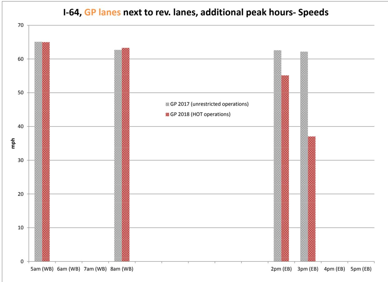
**FIGURE 13 I-64 between Ches. Blvd & Norview Ave- Vehicle Speed, by hour**
