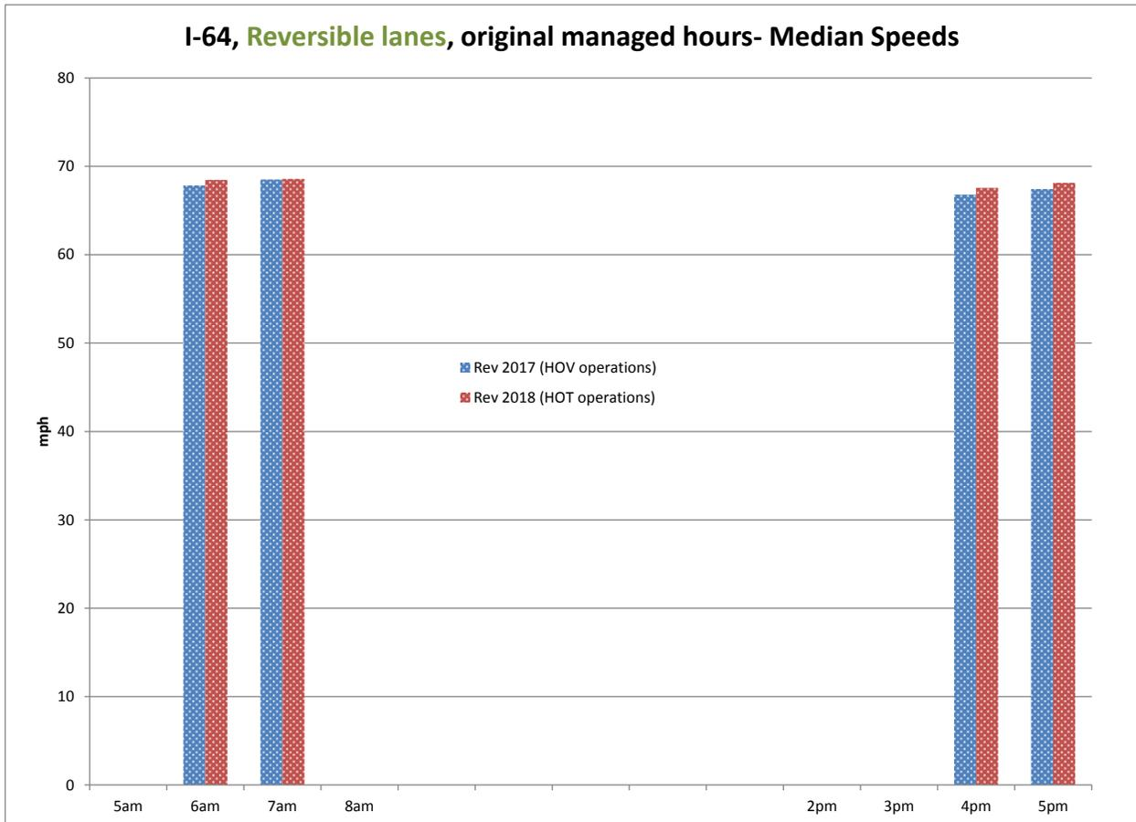
**FIGURE 4 I-64 between Ches. Blvd & Norview Ave- Vehicle Speed, by hour**
