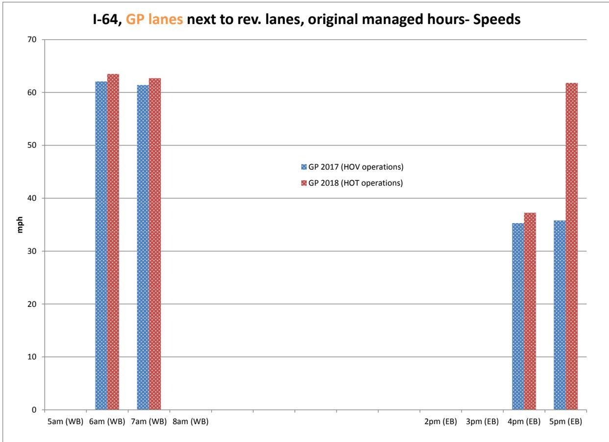
**FIGURE 6 I-64 between Ches. Blvd & Norview Ave- Vehicle Speed, by hour**
