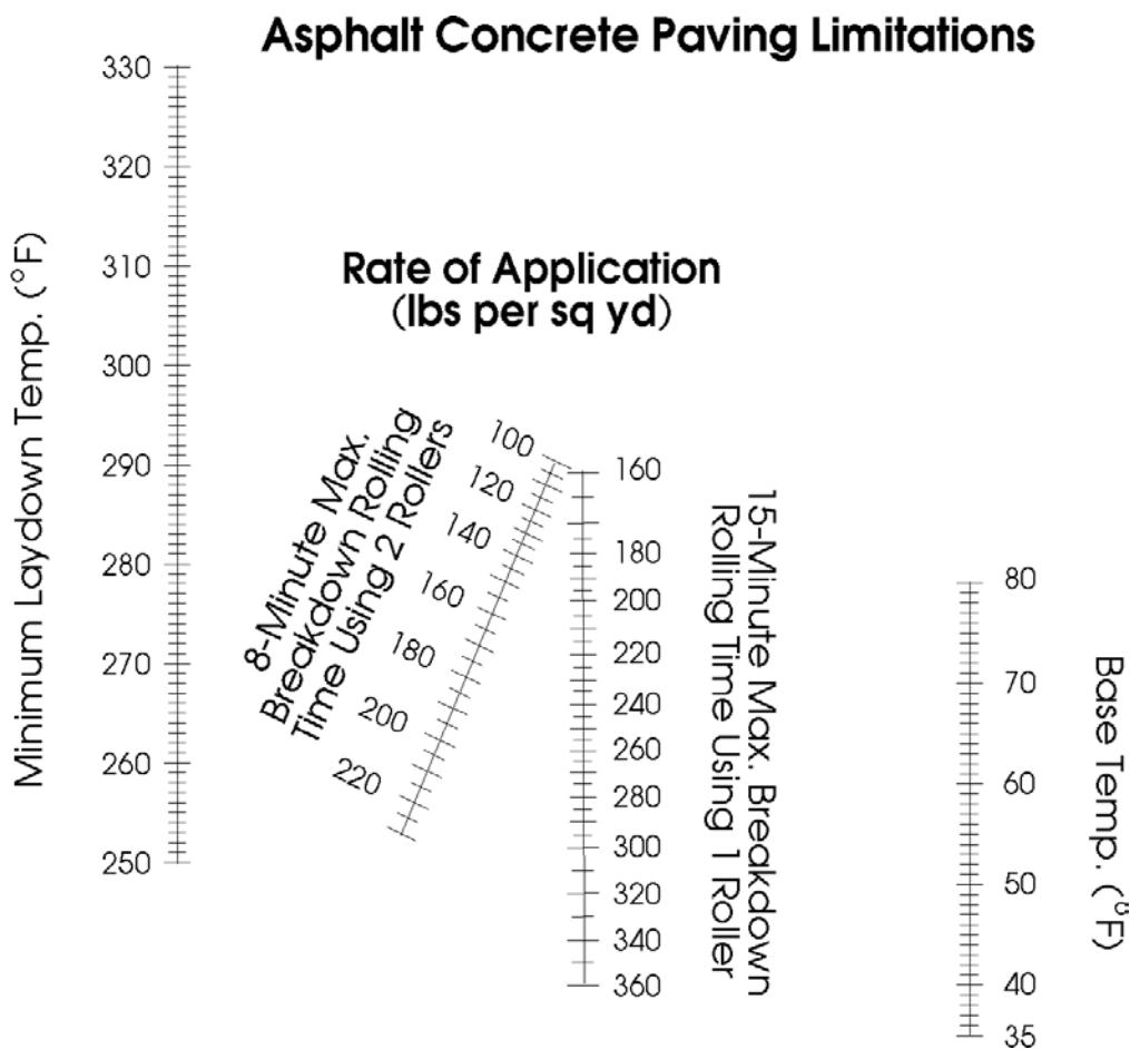
Should the Contractor be unable to complete the compaction rolling within the applicable 8 minute or 15 minute period, the placing of asphalt mixture shall either cease until sufficient rollers are utilized or other corrective action taken to complete the compaction rolling within the specified period.
