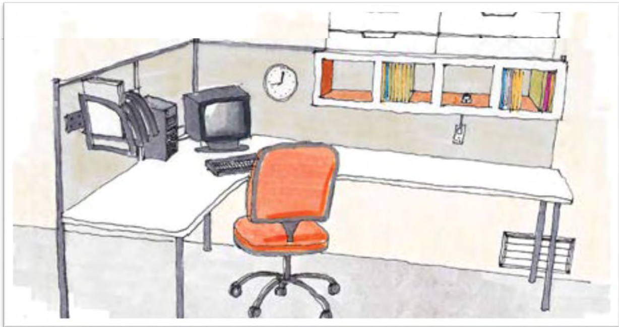
Figure 3. Wet floodproofing a workspace with vents and elevation of equipment. Source: Resilient Industry Mitigation and Preparedness in the City's Industrial Floodplain.
