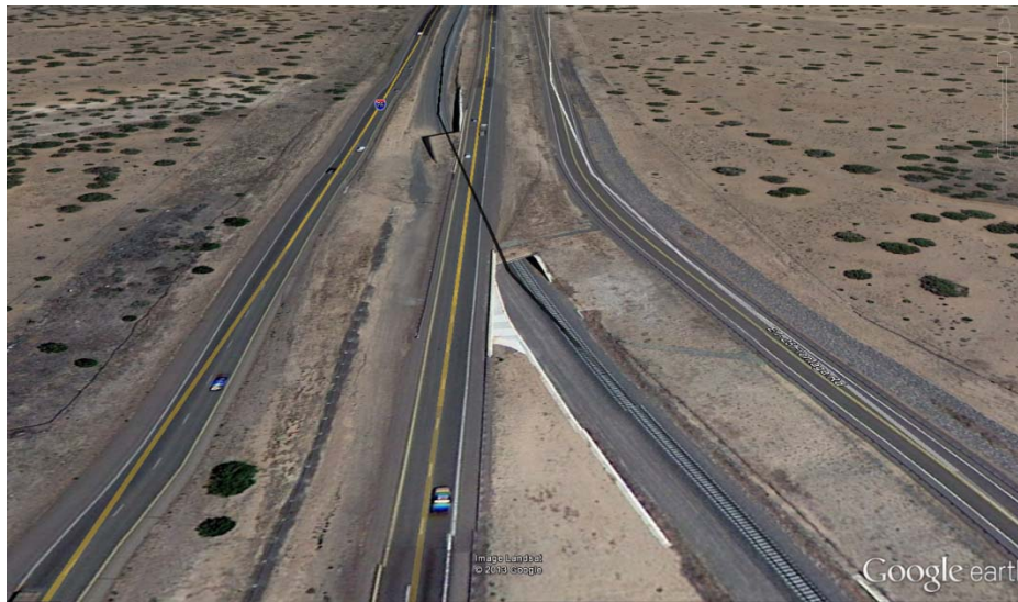
Exhibit 3-13: Rail Line Transition to Interstate Highway Median (near Los Cerrillos, NM)
