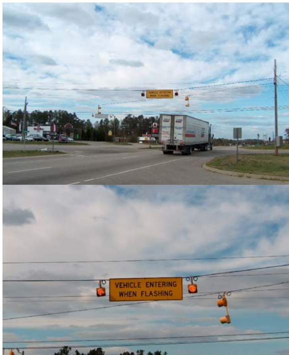
Warning signage used in North Carolina to alert drivers when vehicles are entering the intersection from minor approaches.
