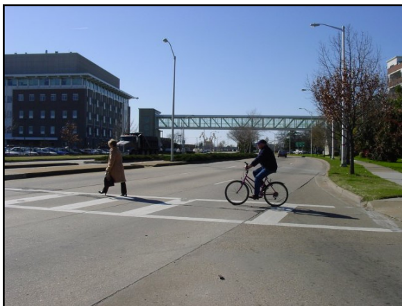
The proposed site for a pedestrian bridge should be at least 600 feet from the nearest alternative "safe" crossing (see third guideline on following page). Here, a crosswalk near the Norfolk hospital pedestrian bridge is about 320 feet away.
