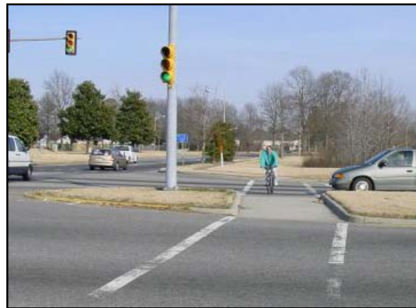
An example of a median refuge island at the intersection of Greenbrier Parkway and Volvo Parkway. Refuge islands allow pedestrians to cross one direction of traffic at a time. They also allow bicyclists to travel safely across the median.
