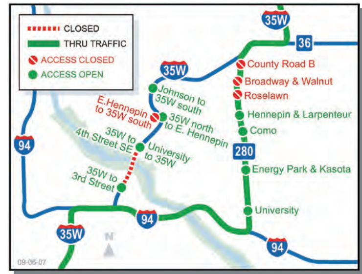
FIGURE 11 – I-35W detour map produced by Mn/DOT. Route 280 was converted to a freeway to handle the diverted traffic. (Source: Mn/DOT.)
