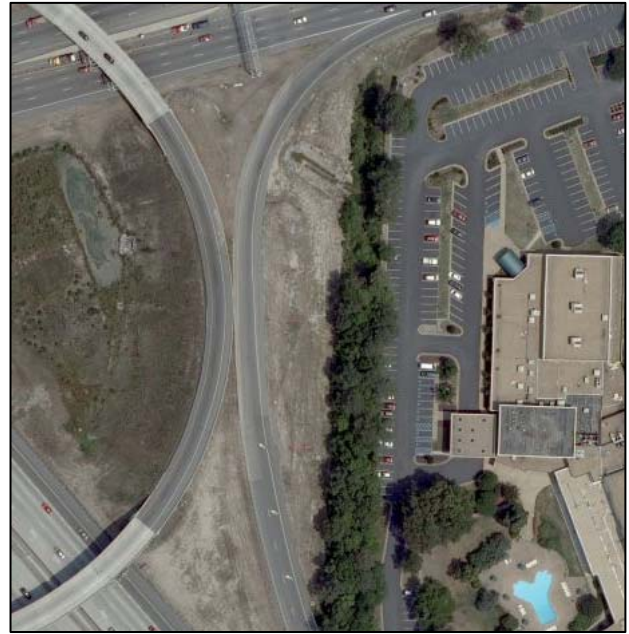
The ramp from westbound I-64 to eastbound Mercury Boulevard drops from two lanes to one before merging with Mercury Boulevard. Aerial image source: Microsoft.
